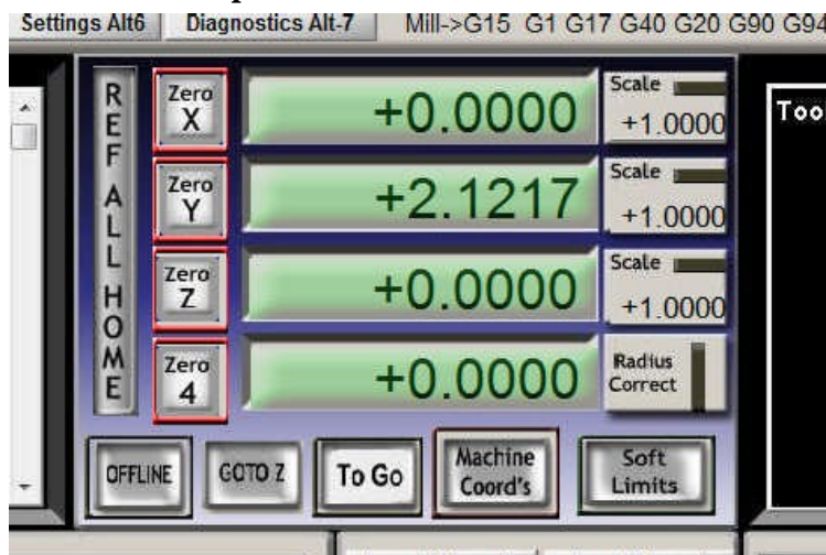
Below is DRO with Spindle 2.1217 inches Forward on Y axis
